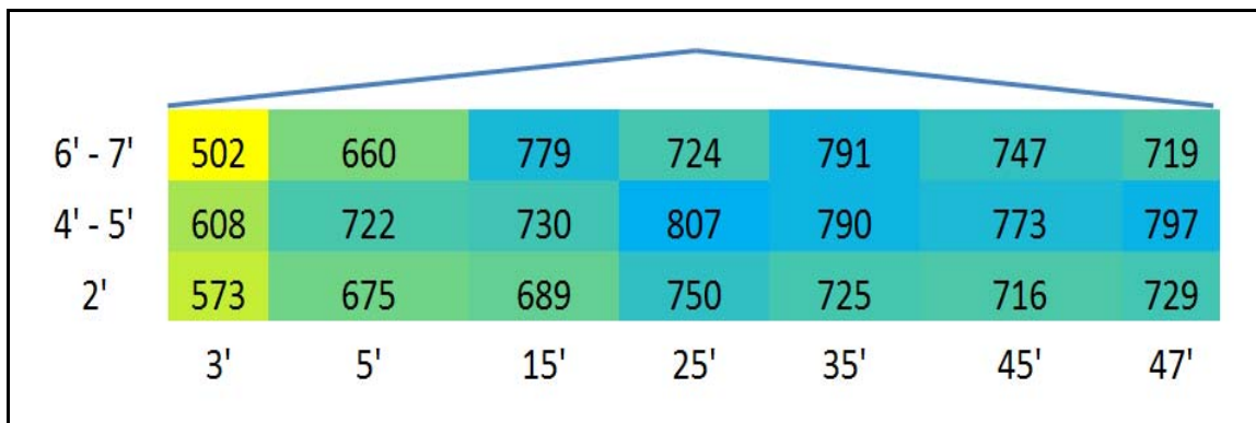
Figure 6. Air velocity profile with forced air furnaces one foot above floor.
