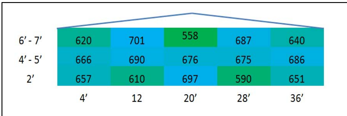
Figure 10. Air velocity profile in totally enclosed 40' wide house with radiant heaters installed at ceiling peak.
