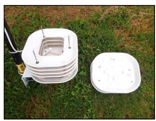
Figure 3. Partially assembled solar radiation shield with temperature sensor (upside down).
