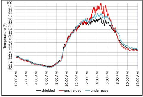
Figure 4. Outside temperature measurements.
