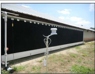
Figure 1. Example of solar radiation shield.
