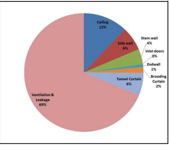
Figure 1. Heat loss from a modern totally-enclosed poultry house.
