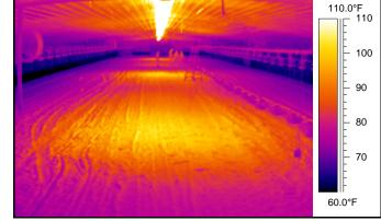
Figure 2. Radiant tube 8' installation height.
