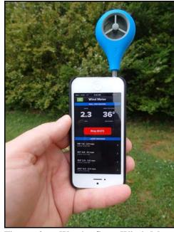
Figure 2. Weatherflow Wind Meter connected to Iphone.
