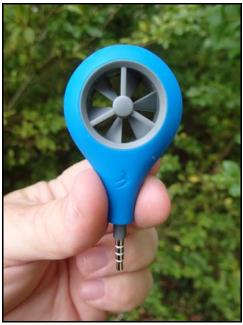
Figure 1. Weatherflow Wind Meter.
