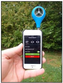
Figure 3. Weatherflow app recording wind speed.
