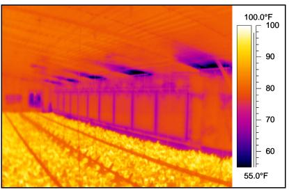
Figure 3. Fresh air entering only through air inlets (very tight house)
