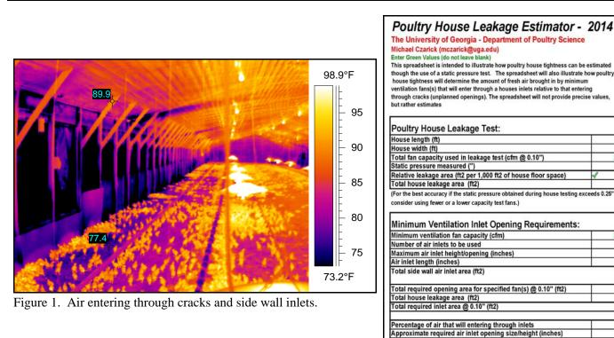
Figure 2. Poultry House Leakage Estimator Spreadsheet
