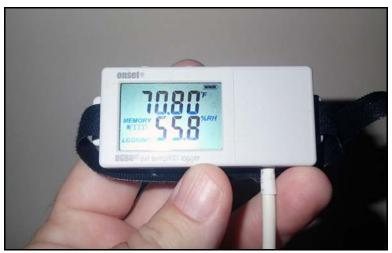
Figure 6. Onset UX100-023 temperature/Rh data logger
