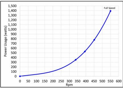
Figure 3. Fan power usage vs Fan speed.
