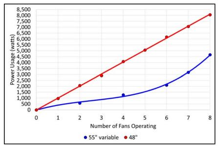
Figure 5. Total fan power usage vs. Number of fans operating.
