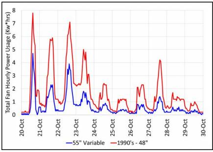
Figure 6. Hourly fan power usage.
