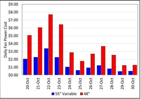
Figure 7. Daily fan power cost @ \$0.10 per Kw\*hr.
