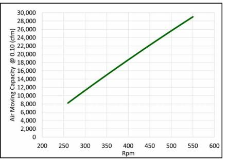
Figure 4. Fan air moving capacity vs. Fan speed.
