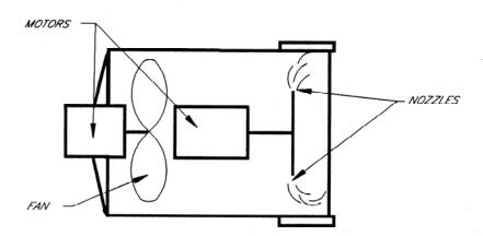
Field application of the fogging-fan is presently being studied by the Extension Engineering and Poultry Science Departments of the University of Georgia. The fogging-fans have been placed in both tunnel-ventilated and curtain-ventilated poultry houses. Preliminary findings show between five and ten degrees of cooling are possible with these units.
