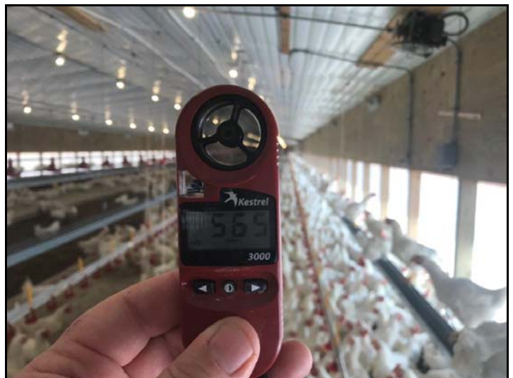
Figure 9. Air velocity 5' from the side wall on the slats (565 ft/min).
