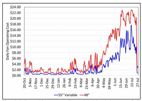
Figure 7. Daily tunnel fan power operating cost in both breeder houses over flock.
