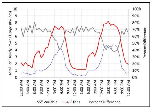
Figure 6. Hourly tunnel fan power usage (May 8 - May 9).
