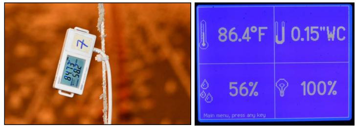
Figure 1. Temperature/Rh data logger
