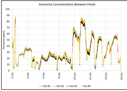
Figure 3. Broiler house ammonia concentrations indicated by the four ammonia sensors between flocks
