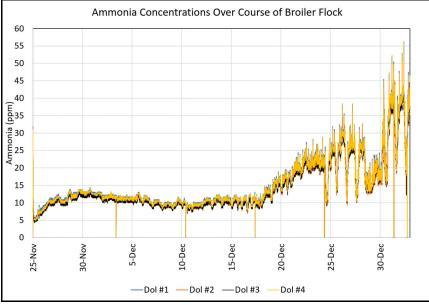
Figure 1. Broiler house ammonia concentrations as indicted by the four DOL 53 ammonia sensors
