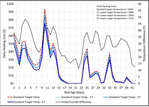
Figure 1. Daily fuel usage and inside/outside temperature difference
