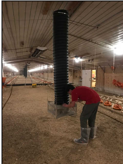
Figure 1. Cubo - vertical circulation fan.
