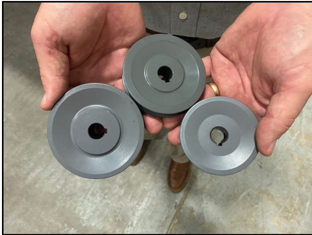
Figure 1. Pulley sizes evaluated (from left to right) AK39, AK34, AK30.
