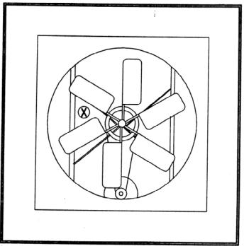
Measurements should be taken at point marked "X" between the shutters while they are held open. Use extreme caution not to get too close to the moving fan blades.
