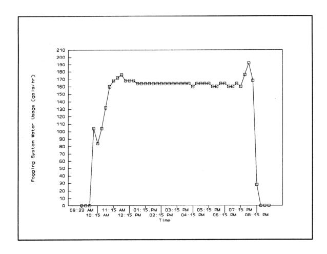
The fogging system in both houses did provide greater than 10°F cooling without excessive house wetting. It was observed during the warmest days that more nozzles probably could have been used without causing any significant house wetting. It appears that in the future fogging systems could incorporate as many as 30, 1 gal./hr. nozzles per fan installed in multiple stage configuration.
