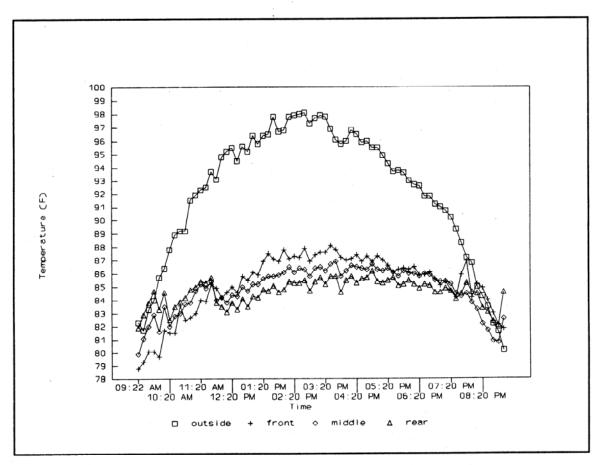
During the second week in July, the birds in the test houses were seven weeks of age. Outside temperatures during this week ranged from the mid 70's at night to the high 90's during the day. On the hottest day, outside temperature reached 98°F with a relative humidity of 45%. During the warmest portion of this day the two-stage fogging system reduced house temperature an average of 11.5°F.
